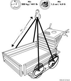
fig. 36 – Anchoring points to lift machine
