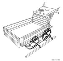
fig. 37 – Anchoring points for transportation
