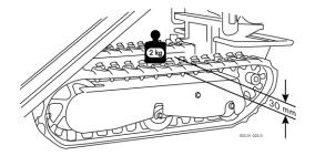
fig. 39 - Check track tension
