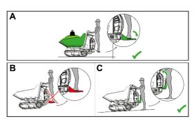
C85 with the platform closed and the operator on the ground.
