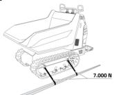
fig. 29- Anchoring points for transport
