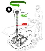
• Press briefly levers driving and control levers; stop the engine and check the oil level on the pin "A" reaches the line of the "MAX" and, if necessary, re- peat the process.
