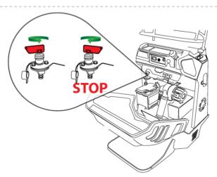
fig. 12– Horn button (above) - Battery switch (bottom)
