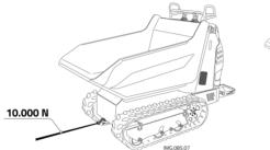
Fig. 28 - Anchoring points for towing
