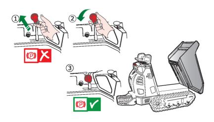
fig. 13 – Parking brake (above) - Throttle (bottom)
