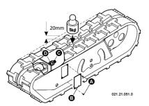
fig. 34 - Regulation track tension
