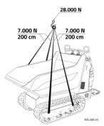
fig. 27 – Anchoring points to lift the machine
