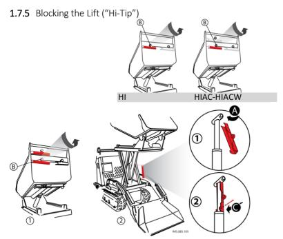
fig. 5 – Blocking the lift
