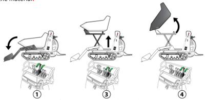
fig. 23 – Position for high unloading
