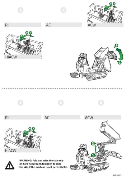
fig. 15 – Lever bucket rotatory (top) Lever Hi - Tip (bottom)
