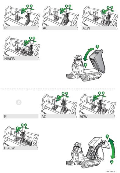
fig. 14 - Dump lever (top) Self-loading lever arm (bottom)
