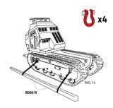
fig. 27 – Anchoring points for transport
