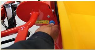
The coasting button is used to disengage the drive wheels, allowing the motorized wheelbarrow to be moved when the engine is off. Turn the button counter-clockwise to disengage. Push the button and turn clockwise to re-engage the engine.
