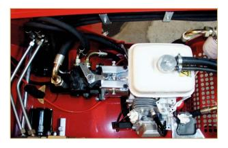
Adjustment - before serial no. 050503-00 Loosen the nuts (1) with a 13 mm spanner. Adjust the nuts (2) until the machine has come to a complete stop. Tighten the nuts (1) again.
