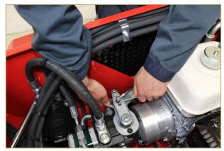
Serial no. 280100-001-2016 and onwards Loosen the lock nut (1) on the underside of the eccentric bolt (2) with a 13 mm spanner. Turn the eccentric bolt (2) to the right or left until the machine has come to a complete stop. Then tighten the lock nut (1) again.
