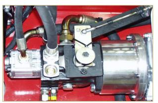
After serial no. 050503-00 to 280100-001-2016 Loosen the bolt (1) with a 6 mm Allen key. Adjust the cable fitting (2) by turning it around the center until the machine has come to a complete stop. Tighten the bolt (1) again.
