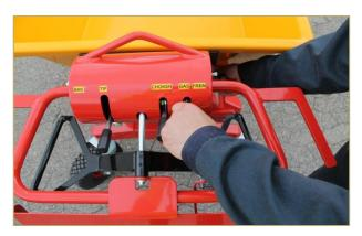
Start the machine by activating the choke when the engine is cold and then turning the ignition key clockwise. When the engine is running, release the key and adjust the choke until the engine is running smoothly. Adjust the throttle to the desired engine revolutions.
