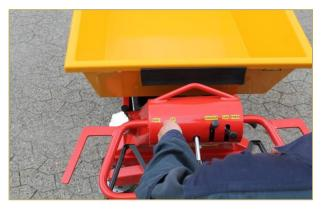
To tip the tray, push the tipping lever up with your left hand, while keeping your right hand on the handle bar. Use the lever to adjust the speed: the more you push it, the greater the speed.
