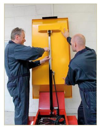
While one person holds up the tray, the other mounts the safety fitting on the hydraulic cylinder.
