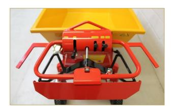
Pressing the safety plate should move the machine forward, preventing the operator from being trapped during reverse.
