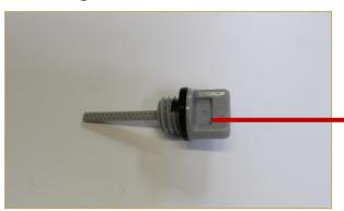
Oil must be visible on the dipstick or top up with type SAE 15W-40 engine oil, if necessary.
