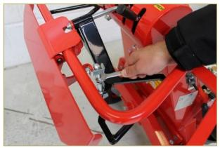
Loosen the two lock nuts with a 13 mm spanner. Remove the cotter bolt from one angle joint, and remove the head from the ball. Now turn the angle head in or out as required.
