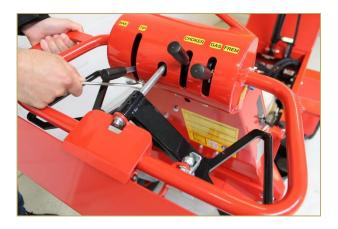
Adjust the stop so that the tray is lowered at a steady speed, but the engine does not sound strained.
