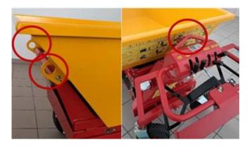
Ensure sufficient stability during lifting to prevent disconnection.
