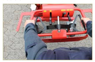
Place both hands on the handle bar so that your fingers can reach the forward handle. Pull up the hand lever on the right to move the machine forward and release to stop. Pull up the hand lever on the left to reverse.
