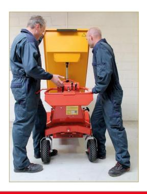
In case of an engine fault, the tray can be tipped manually.
