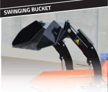
The swinging bucket not only load the dumper but can unload it frontally
