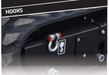
Large and sturdy hooks to move the machine in total safety.
