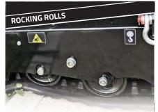
The machine's undercarriage oscillated to follow the terrain profile for increased stability and comfort.
