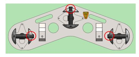
Step 2: Check that the glass sucker is level using the spirit level Reposition the glass sucker until both bubbles in the spirit level are inbetween the two lines. This will indicate that the glass sucker is level.
