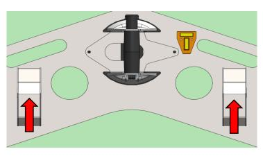
Step 5: Insert the fork tines securely into the pick-up bracket
