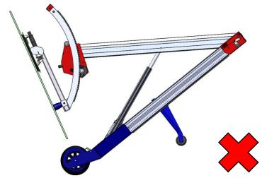
2) Do not lift glass panel, if the red line is still seen (the glass panel is not properly secured onto the glass sucker).
