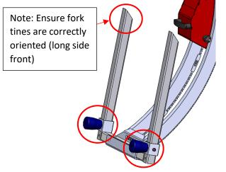
Step 5: Pickup brackets indicated in the diagram below
