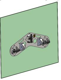
Step 3: Press the three suction buttons on the glass suckers to lock onto the glass panel
