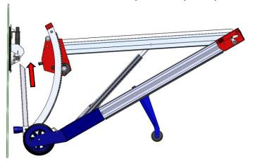
Step 5(Continue): Insert the fork tines securely into the pick-up bracket
