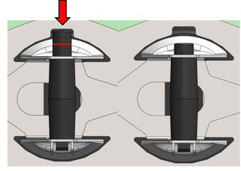
Step 4: Slide the two rubber spacers into the fork tines and tighten the bolts
