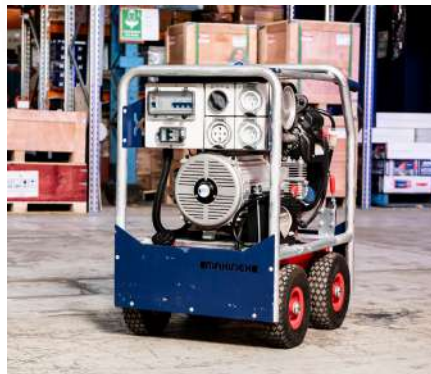
2. Power Generator 16 kVA
