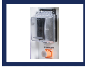
4. AC and PV Charging Inputs
