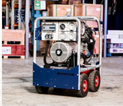
2. Power Generator 16 kW
